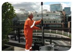
For medium and long term noise monitoring applications, the Invictus can be combined with a secure enclosure for wall or mast mounting. Its large, clear colour touch screen allows the instrument to be deployed quickly whilst allowing the user to see the exact status of the system.
